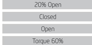
The display shows the position of the valve as a percentage of opening when it is partially open. The display shows "Closed" when the valve is closed. The display shows "Open" when the valve is open. The display is factory set to show the instantaneous torque as a percentage of the maximum actuator torque value < 10% indicates the minimum torque value.
