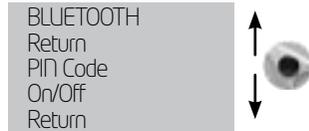
The PIN code can be modified. This code will be requested when attempting to connect to the actuator. On/off allows to activate/desactivate the Bluetooth connection. This option is 'on' by default and is not memorized in case of actuator reboot.
