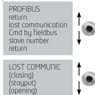
**Bus control:** Bus control is normally selected. For equipment which also uses a standard hard-wired system, this configuration allows the user to choose the command mode: either via bus or hard-wired (see §7.1 and §7.2)
