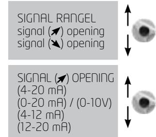
With 0-10 V signals, two contacts are also switched to OFF. The contacts are located on the INTELLI+ board (supporting the display) inside the control unit.
