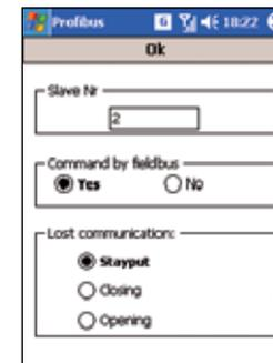
If a Profibus interface is detected on INTELLI+ by INTELLIPOCKET, the configuration window is available with the "Check/Bus" menu or "Change/Bus" menu. The following window is displayed.
