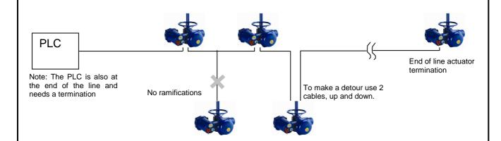
Maximum line length is 1200m (3600ft). Maximum number of actuators by line is 30. Maximum line length is reduced according to the communication speed.
