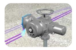
Fieldbus is advantageous because it allows getting more information while reducing the overall wiring on site. However, when you break up the continuity of the line, for instance because of one actuator being retrieved from the field for maintenance, your whole installation is affected since the signal cannot circulate anymore.
